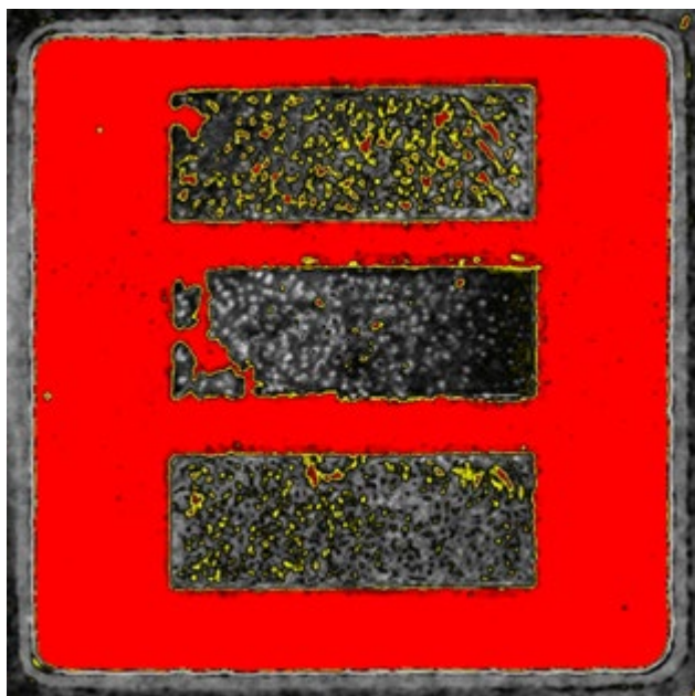
Figure 3: The three die in this power discrete device have voids in the die attach.
